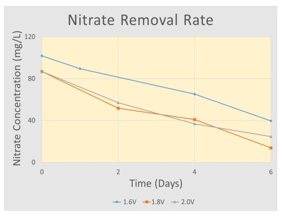
Figure 5: BER nitrate removal rate
